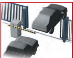
automatic p.a.m.s. sequencing with slide and swing gates
